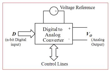
The only register specific to the DAC that we use is the **DACR** register, shown here. On the LPC1768 the reference voltage is applied between terminals labelled  $V_{REFP}$  and  $V_{REFN}$ ; these are connected to 3.3 V and 0 V respectively.
